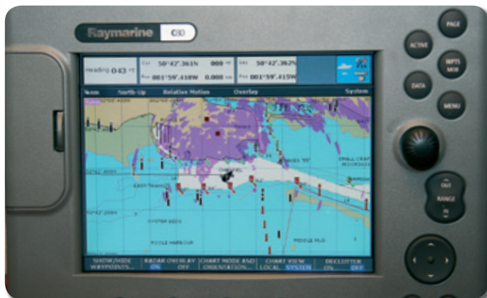
The radar image overlays the chart in pink, newer sets offer this useful feature.
